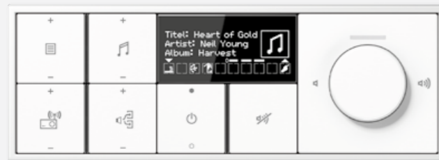
Combined operation of multirooming and classic room features with KNX controls.
